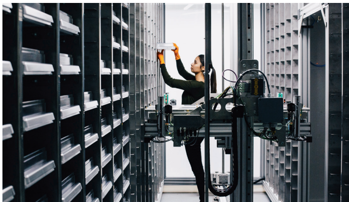
GESA the robot removes the germination trays from the store, photographs the germination progress and returns them to the shelf.
